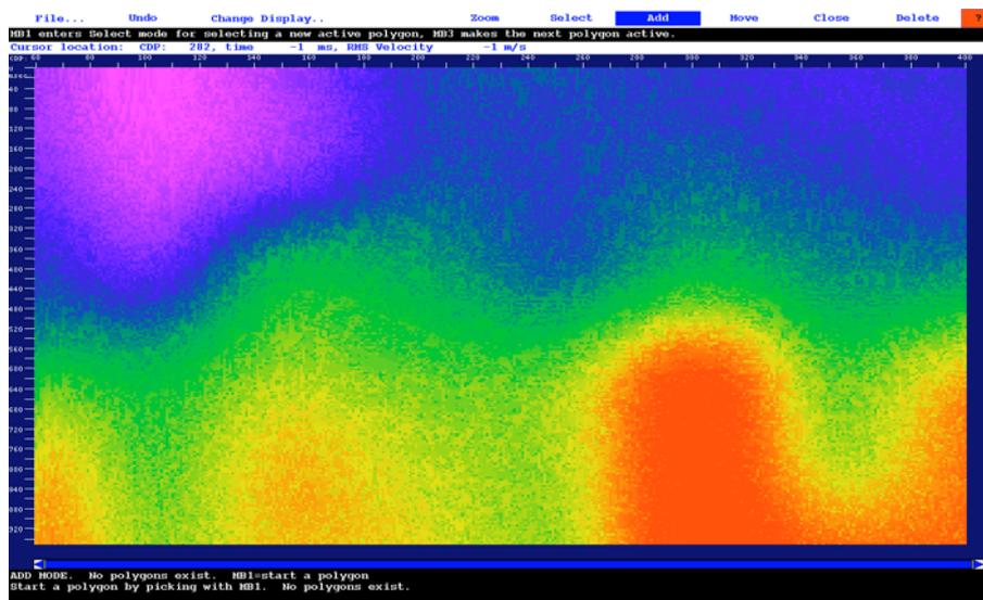
Fig. 2 Stacking velocity from CRS velocity search
