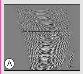
Specularity Gathers show the illumination angle at each depth location with reflections curved and diffractions flat (A). After eliminating all reflection energy (curved) from the Gathers the diffraction Energy remains and can be stacked (B).
