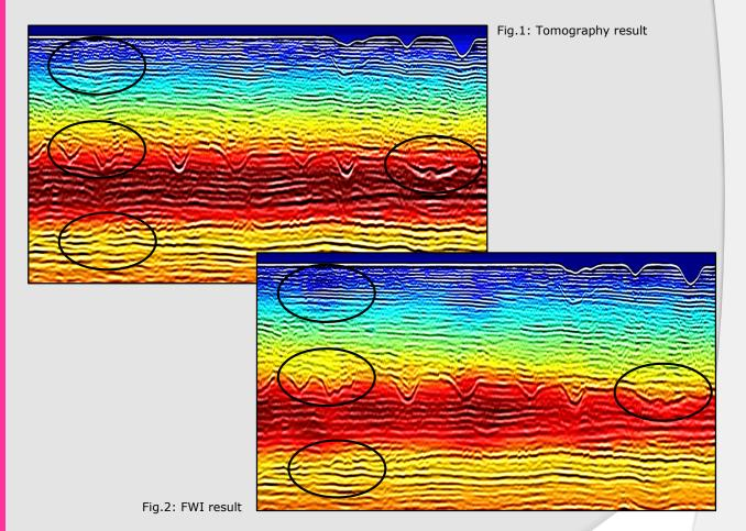
The example shows a tomography (Fig.1) and a FWI result (Fig.2), respectively. The FWI model has a better resolution (low velocity zones in the upper part, channels in the lower part). The overlaid RTM image benefits from the improved velocity model.
